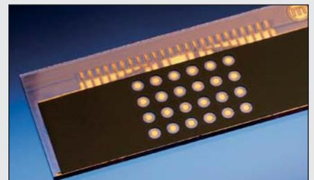
Nano Well Plate with 24 individual contact wells. The excimer laser ablates the electrodes from a gold layer as well as the holes in the foil. The wells have a diameter of 2,5 mm and a depth of 150  $\mu\text{m}$  (intervals 3,8 mm)
