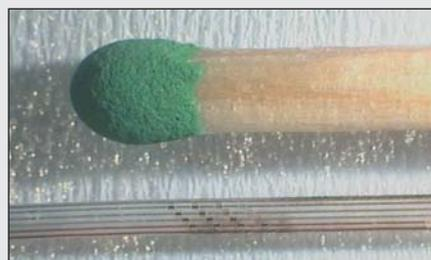
The accurate stripping of micro wires is achieved with the excimer laser. A major advantage is the non-thermal ablation of the isolating material, since the plastic material does not melt. Materials used for isolation: polyurethane (picture), polyimide and others
