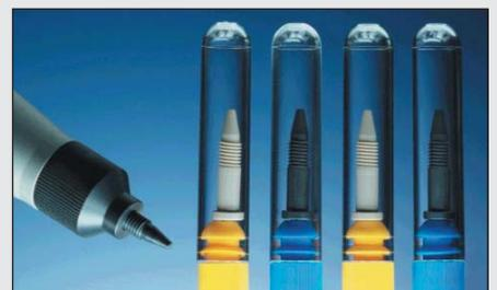
The CryoPen® freezes tissue in the cryo therapy without destroying the fibre structure. The decisive part of the CryoPen® is a micro nozzle made of PEEK. The excimer laser drills a hole of 30  $\mu\text{m}$  in diameter into the tip. Compressed laughing gas (N<sub>2</sub>O) cools down to -89°C (Joule-Thompson-effect). The CryoPen® is manufactured by Bartels Mikrotechnik for H&O Equipments.
