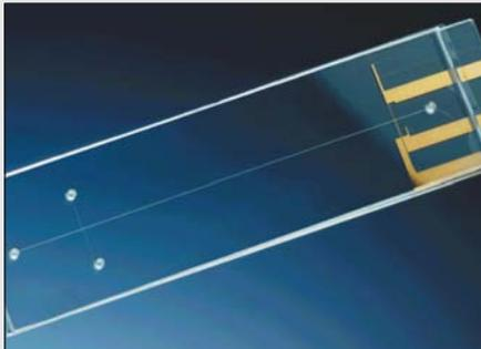
Capillary electrophoresis is a strong separation tool for biotechnological applications. This "lab-on-a-chip" is made of polycarbonate. The channels of 50  $\mu\text{m}$  width and depths ranging from 20 to 50  $\mu\text{m}$  have been created with an excimer laser.
